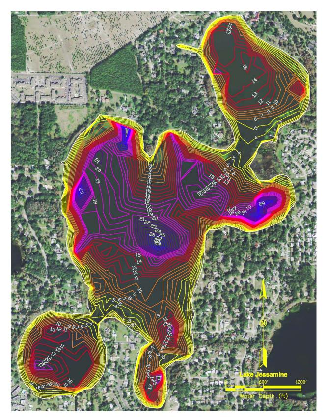
Figure 1-4. Water Depth Contours (ft) for Lake Jessamine on March 29, 2011. (Water Elevation = 89.84 ft).
