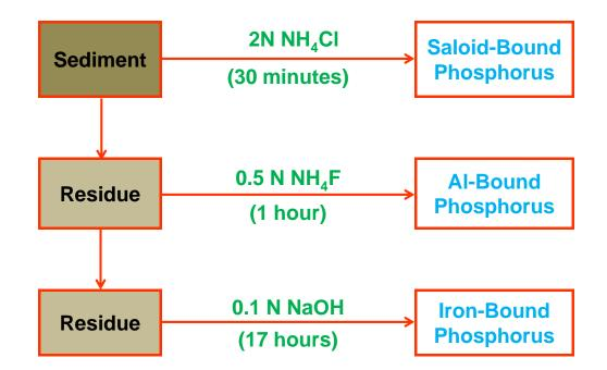
Figure 2-2. Schematic of Chang and Jackson Speciation Procedure for Evaluating Soil Phosphorus Bonding.
