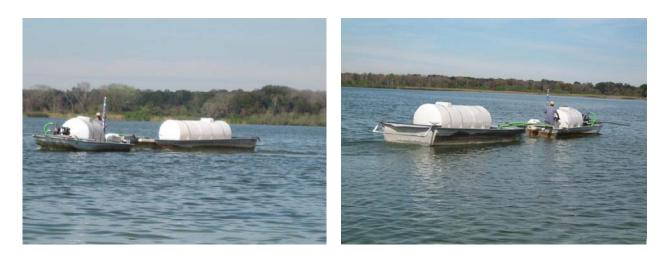
Figure 2-5. Application Boat and Tanker Barge Used for Alum Application in Lake Jessamine.
