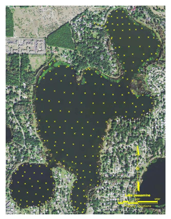
Figure 1-3. Probing Locations for Water and Muck Depths in Lake Jessamine (March 29, 2011).
